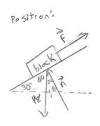
4) A 20 kg box rests on a ramp that is inclined  $18^{\circ}$ . Resolve the weight into rectangular vector components that keep the box at rest.
